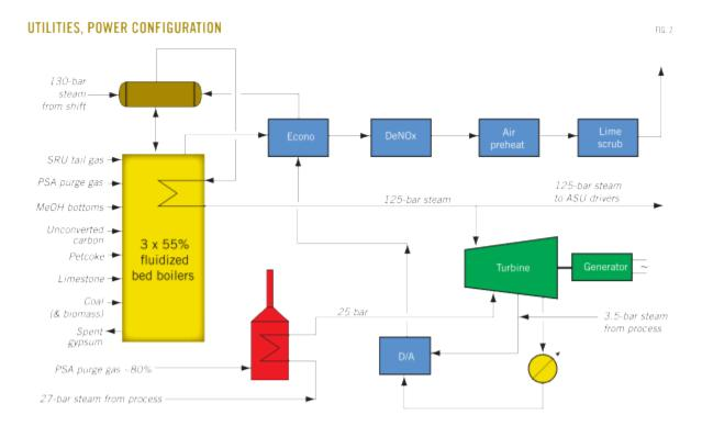
Note that the utilities' consumptions and balances are based upon summer conditions, with 25° C. ambient temperature. Fig. 2 provides a flow scheme of the steam and energy systems.
